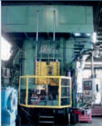
Hydraulic press Cycle time: 7s Pressing force: 400 tons
