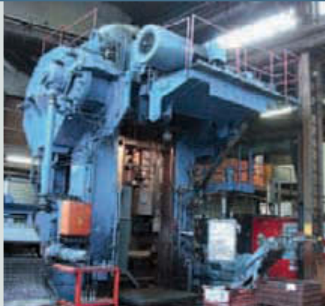
Eccentric press Cycle time: 2.5s Pressing force: 1,600 tons
