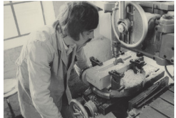
Milling a plastic model in the die shop in 1976
