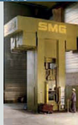
3-stage manual cold press Cycle time: 8–10s Pressing force: 1,000 tons
