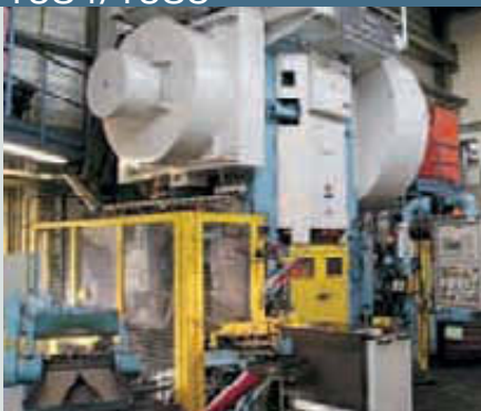
Crank press, fully automated Cycle time 2.5–6s
