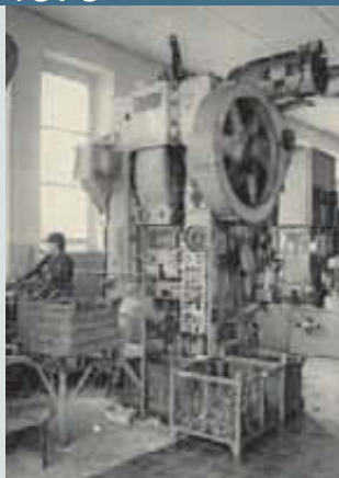
1-stage manual cold press Cycle time: 8–10s Pressing force: 400 tons
