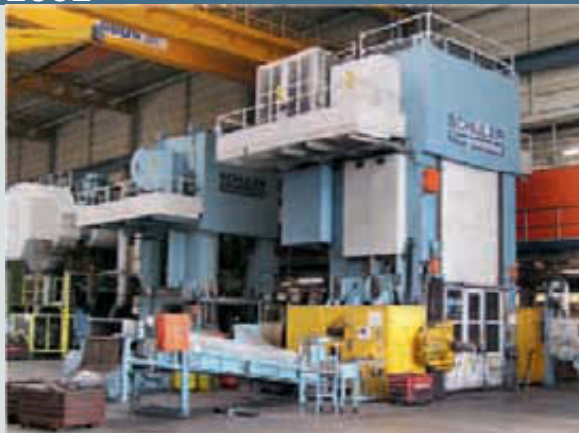
Eccentric press Cycle time: 2.5s Pressing force: 2,000 tons
