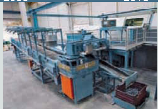
Horizontal, mechanical multi-stage press Cycle time 0.8–1s
